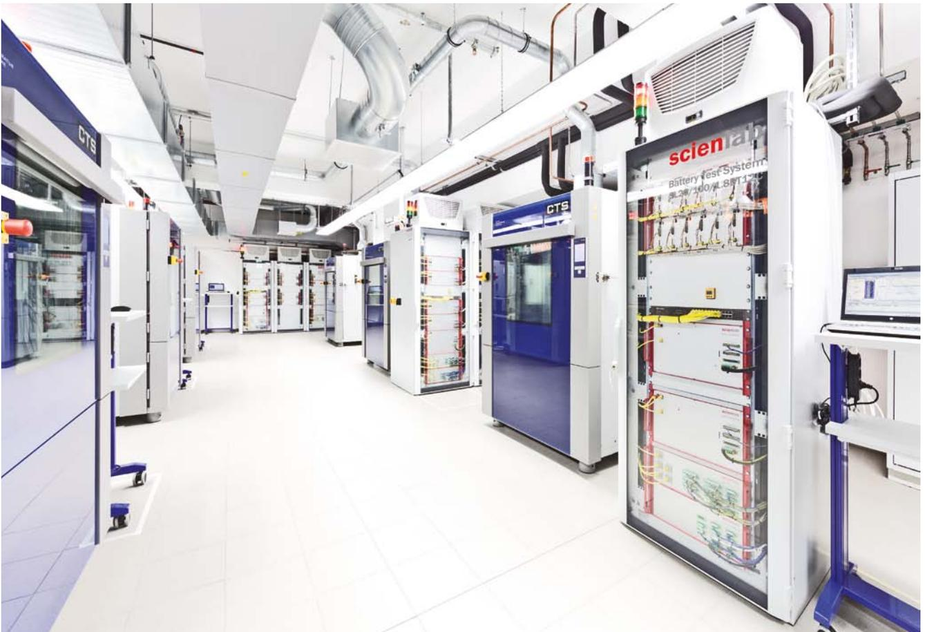
Scienlab test bench for characterization and development of battery cells and modules
