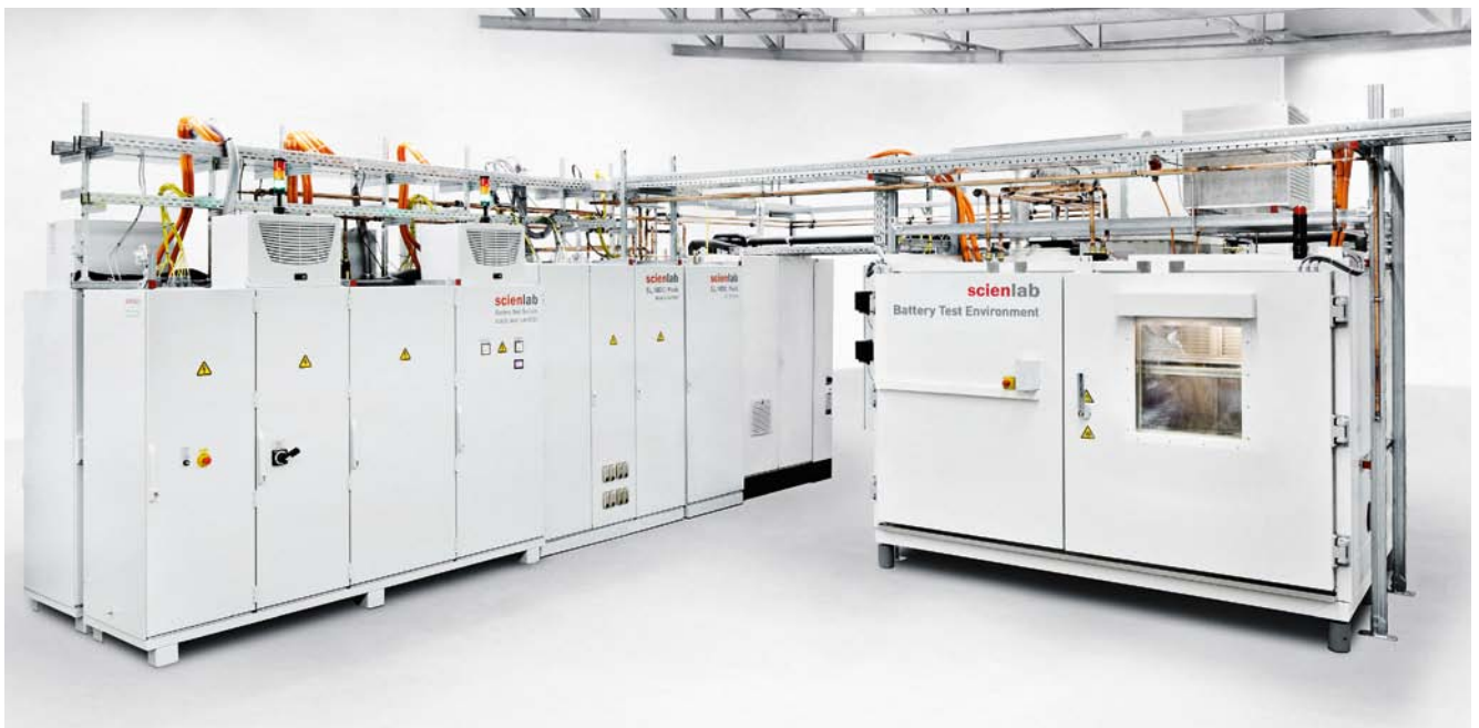
Scienlab test bench for validation of battery packs
