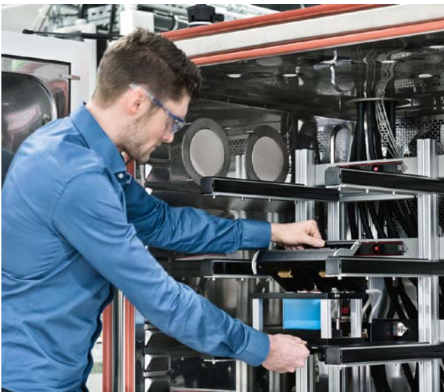
Contacting of a battery cell in the climate chamber
