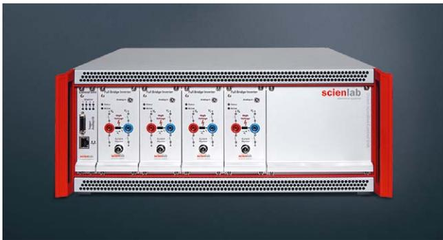
Direct Injection Control Unit (DICU) – electromagnetic
